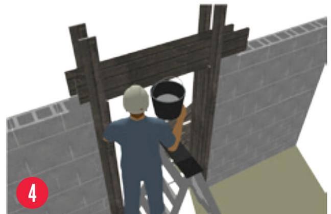
Completion of lintel after steel reinforcement and pouring of concrete
