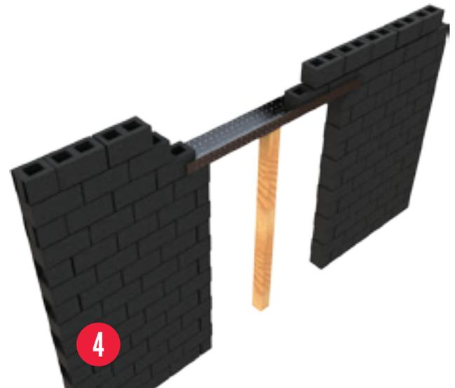
Before laying the blocks down on lintel, place a temporary support beneath the lintel to provide support and to prevent deflection. Temporary support can be removed after the mortar sets, (approximately in 3 to 5 hours).
