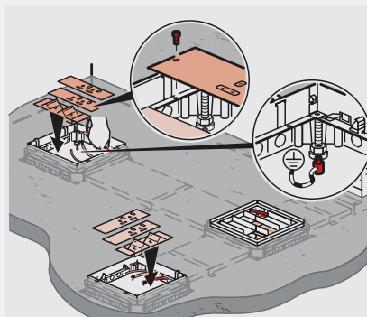
8- Connect wiring and fix the wiring accessory plates onto the backbox. Earth the system
